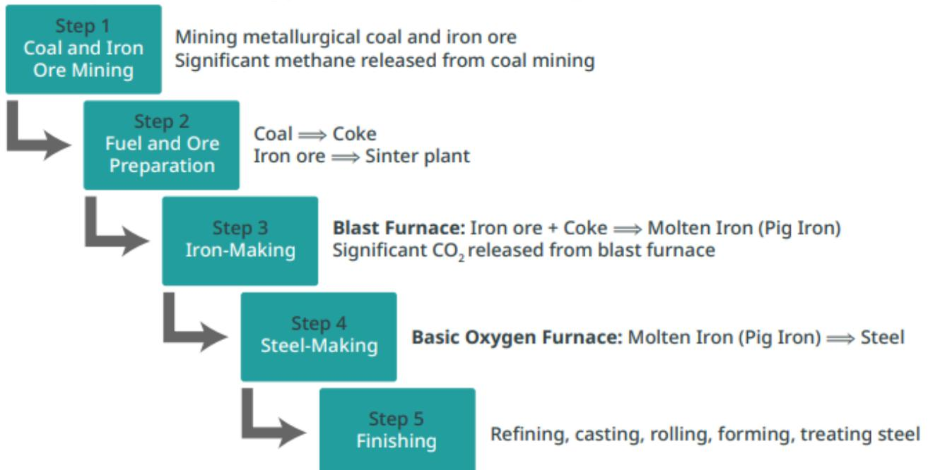
*The 5 steps of conventional coal-based blast furnace steel production. Source: SteelWatch*
